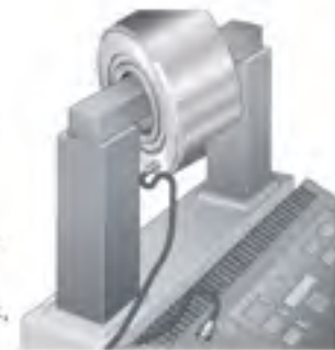
Heating with an induction heater
